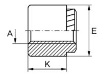
Female thread A = M2,5 Height K = 3 Hole diameter +0.1 = 4.2 Min distance to edge = 2.4 Min material thickness = 1.5 Outer diameter E = 6
